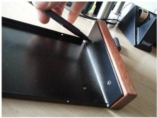
5. Drill the supplied screws vertically into the markings. It's not necessary to drill them completely to the end. This step makes it much easier finding the position and drilling the screws in by hand later. You should drill the screws out again auf course :-)
