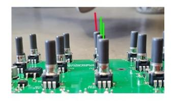
If you are sure each pot is perfectly vertical you can put the pcb on the table with the pot axis facing down and start to solder the middle pin of each pot. Then check all pots again. It also makes sense to lay the pcb into the upper half of the steelcase for having a look with another reference.
