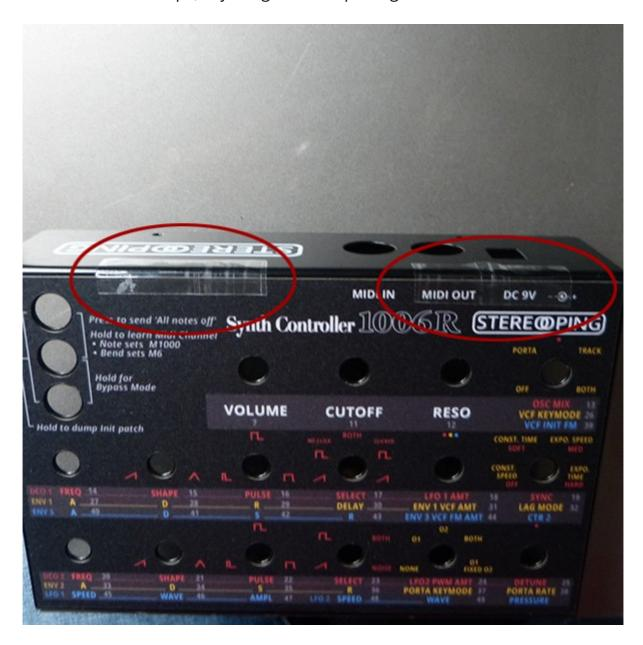
4. The most important position are the 3 holes in the upper left. They will not be covered by knobs later and have to match 100%. Well, all in all it's an optical problem, the controller will work perfectly even with a slightly twisted faceplate.
