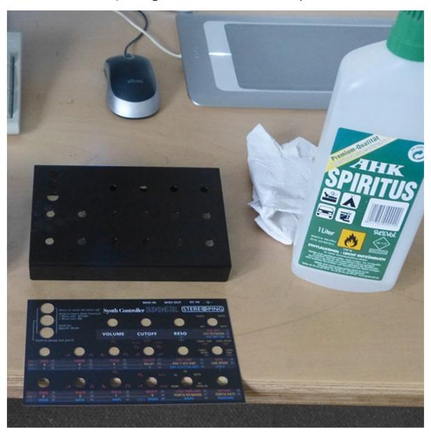
2. Adjust the Faceplate for the 3 drillings and the bottom-right-most hole to fit exactly the case's holes.
