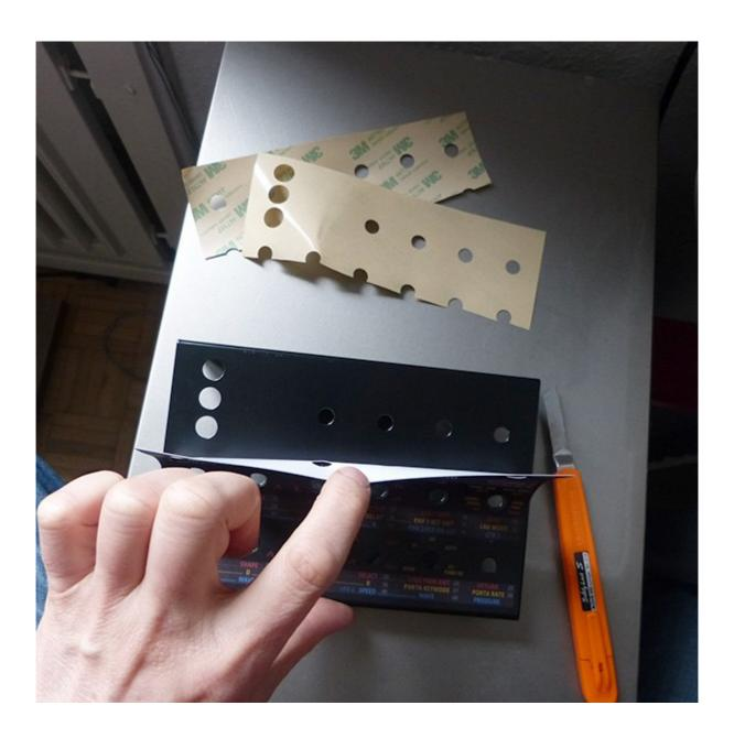
9. Use the slippery backside of the protection foil to press the faceplate onto the case without making it greasy by your fingers.
