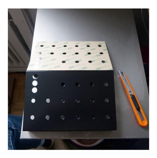
Synth Controller - Sticking Faceplates V1.1 - 03.2015 © Stereoping Germany, Hattingen 2015 6. First remove the bottom part of the protecting foil and cut it off. It's not important to cut a perfect line. Swing the Faceplate back, **do not press it on the case yet**. Check if the sticker still sits where it should. The faceplate is a bit bent concave preventing it to stick itself to the case, you still can adjust the position.
