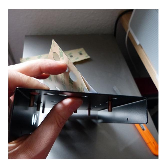
8. Remove it and gently press the faceplate on the case from the middle to the edges. Try to avoid touching the adhesive areas if possible, especially around the 3 buttons. This area will be touched a lot during the years of usage and should stick on the case as perfect as possible.
