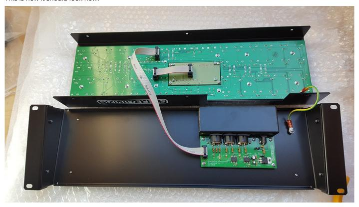
Now you can put both halfs of the case together. Mind the ESD and the flatcable to fold nicely together when attaching the upper half. It would not be good if one or both got clamped between the case parts.
