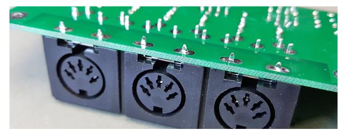
Preferably there should not be any space between jack and PCB. Otherwize take PCB and jack between thumb and trigger finger and heat up the single solder mark again. The jack will snap into optimal position.
