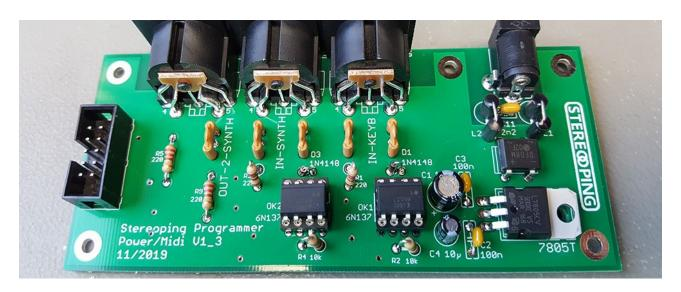
One little word: if you got the PCB laying in front of you like on the picture above, the optocouplers will be plugged into the sockets upside down. Therefore another detail picture:
